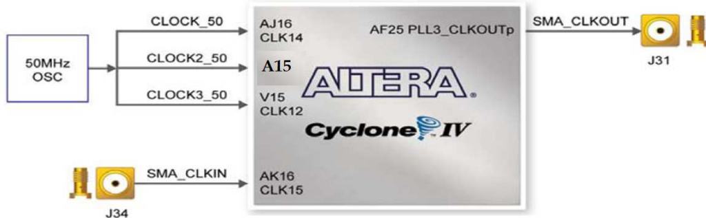
Block diagram of the clock distribution
